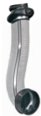
The tension of a leaf spring in the hose holds the nozzle firmly to the exhaust pipe. The spring also ensures the release of the nozzle when the electro-magnet is deactivated.
